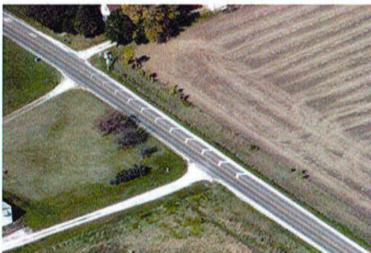
Figure 5. Experimental converging chevron markings followed by "25 MPH" pavement legend.
