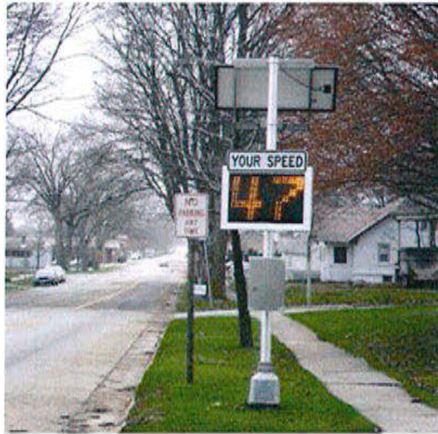
Figure 2. Speed feedback sign in Union.
