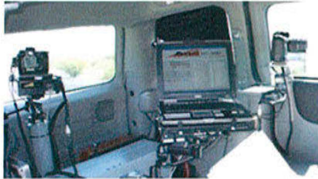
The equipment within an automated speed enforcement van.
