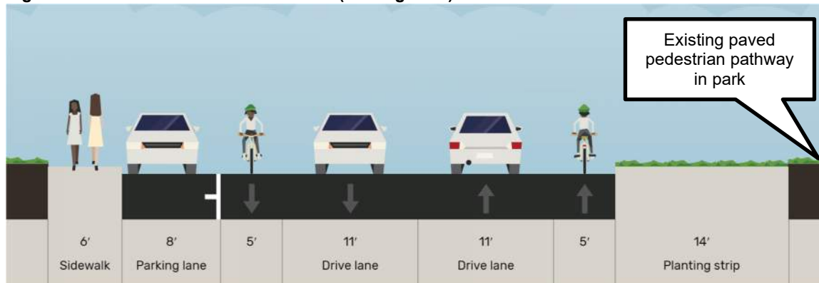
Figure 4. 36th Street E Cross Section (looking west)
