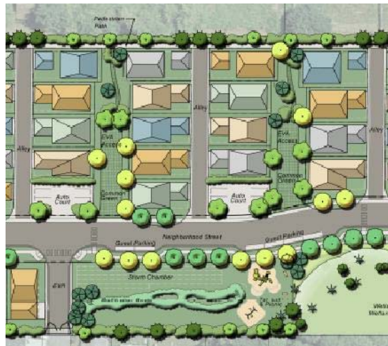
Figure 61 – Site plan for cottages oriented around common greens with alley access for vehicles. Pedestrian connections are provided through common greens and designated pedestrian paths.
